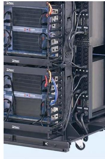
**Figure 5. POU mounting locations help keep air exhaust pathways behind servers clear to provide maximum airflow and enhance equipment cooling.**
